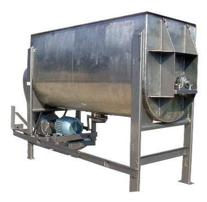
It is an equipment used for mixing solids along with other solids as well as liquids; The Unit Consists of U- Shaped horizontal trough and a specially designed double helical ribbon agitator rotating within. Ribbon Blender provides high degree of mixing in less time with efficient blending.
